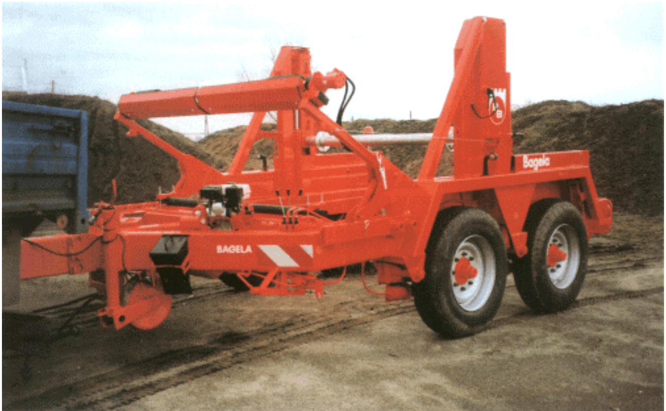
BTT 140.25 with power hydraulic drum drive and lifting system
